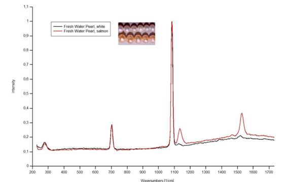
The GL Gem Raman can be used to detect treatment of freshwater cultured pearls: all natural colour pearls show the two major Raman resonance features of polyacetylenic pigments assigned to C=C stretching at about 1530 cm<sup>-1</sup> and C-C stretching at about 1130 cm<sup>-1</sup>.
