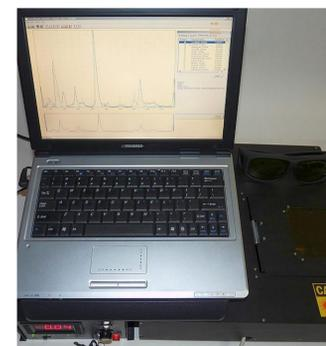
The GL Gem Raman quickly can tell the difference between diamond, cubic zirconia, glass and zircon, distinguish jadeite from nephrite, separate real from faux pearls, tell whether it is ivory or plastic.
