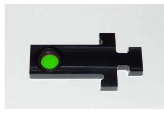
Recently (June 2014) the removable GL Gem Raman Band Pass Filter™ (GLBPF) for suppression of fluorescence in Raman mode has been introduced. In combination with the TEC option useful Raman signals can be measured in strongly fluorescent samples which was almost impossible with basic Raman spectrometers before.
