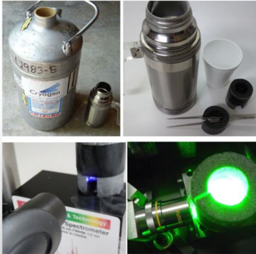
Low cost LN (liquid nitrogen) Accessory (Prototype)
